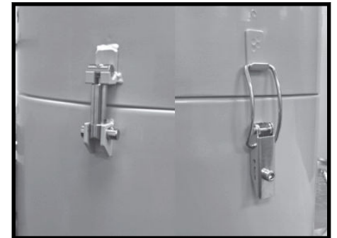
Step 18. Re-assemble unit. Ensure safety latch and clip are securely fastened.
