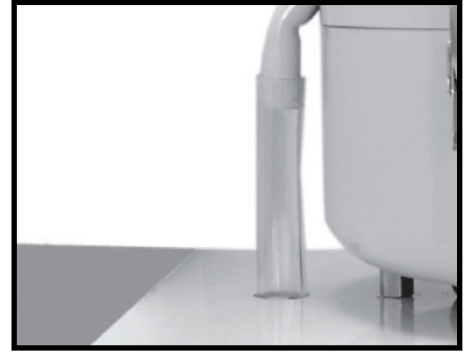
Step 3. Check the oil return hose for damage and blockage.
