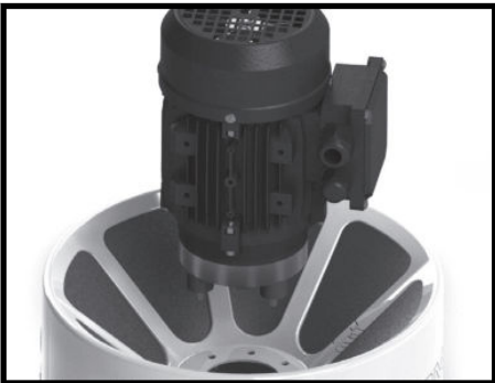
Step 10. Withdraw motor from housing.
