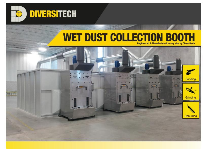
Diversitech's Wet Dust Collection Booth offers a simple, customizable and turnkey solution to handle combustible dust collection for larger work pieces. The stainless steel Wet Dust Collectors serve as the booth's filtration system, and range in size from 3000CFM, 5000CFM, and 6500CFM units. A standard auto-level water control system works to reduce maintenance and increase your production uptime
