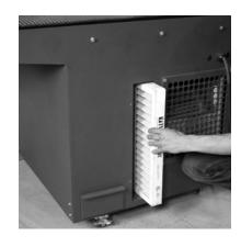
6. Ensure airflow indicator points in correct direction.
