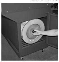
2. Unscrew twist knob to release the filter.
