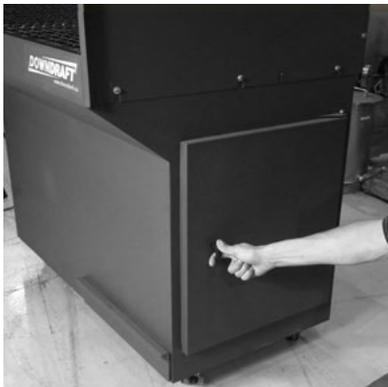
2. Unscrew twist knob to release the filter.
