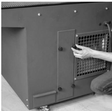
2. Remove Metal Mesh Prefilter (if applicable).
