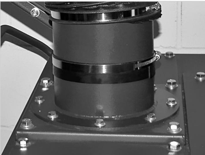
**STEP 2.** Attach swivel base to mounting plate.
