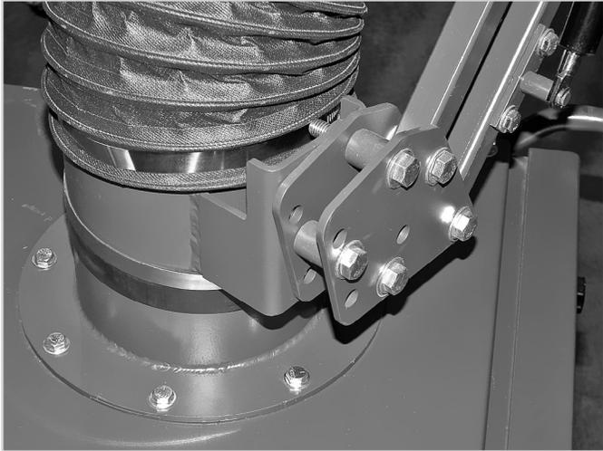
**STEP 3.** Attach capture arm to swivel base.
